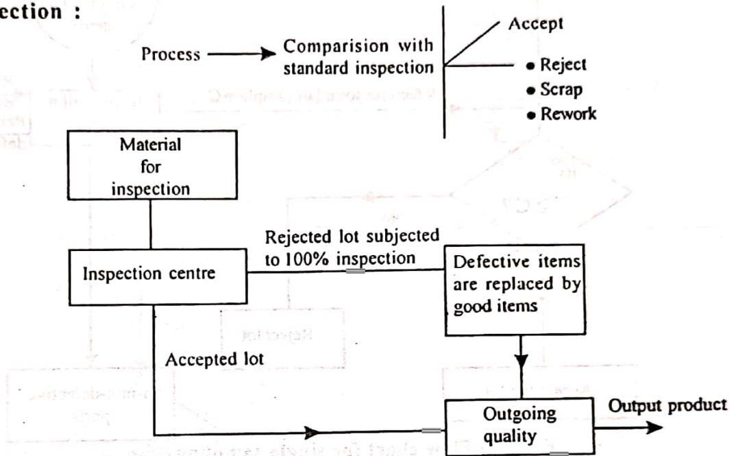
**Fig.2.27 Principle of sampling inspection in any process.**
